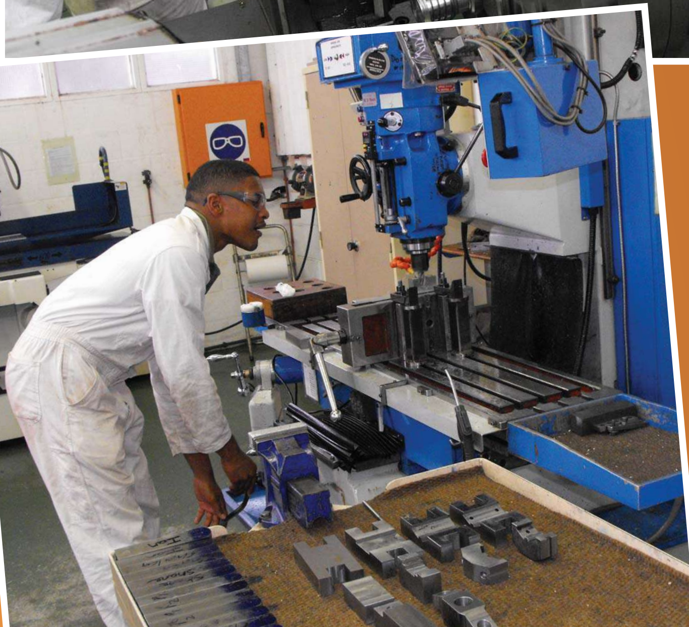
Top: Shane Bowles machining a left-hand square thread. Bottom: Macneal Samuels milling components for his pipe-vice project.
