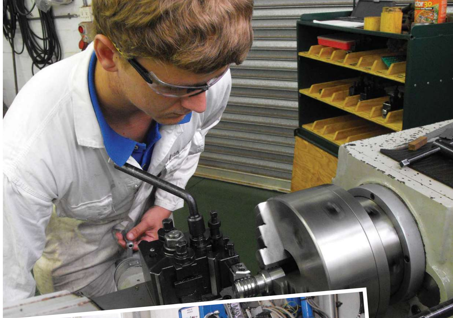
Top: Shane Bowles machining a left-hand square thread. Bottom: Macneal Samuels milling components for his pipe-vice project.
