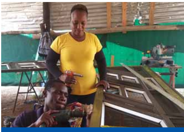
Matlhamela with Tshilisanani Rakhutsi, putting hinges on an aluminium door.
