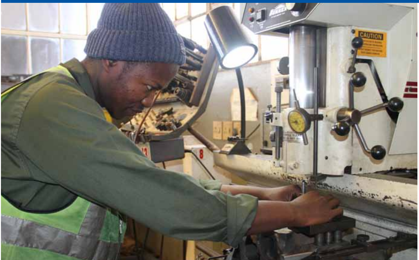
» Chomane reconditioning a cylinder head
